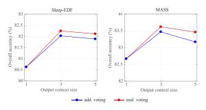
Fig. 8. Influence of the output context size to the overall accuracy of the proposed framework. The results obtained with a common Q=1000, in addition, P=2 (Sleep-EDF) and P=3 (MASS).
