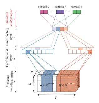
Fig. 3. Illustration of the proposed multi-task CNN architecture. The convolution layer of the CNN consists of two filter sets with temporal widths w=3 and w=5. Each filter set has two individual filters. The colors of the output layer indicate different subtasks jointly modelled by the network.
