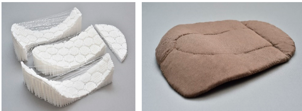
Figure 13. Final product of 3D printing of human body shape.
