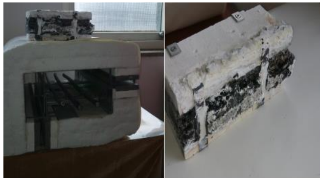
Figure 1. Ceramifiable IFR protector and the IFR protection effect.
