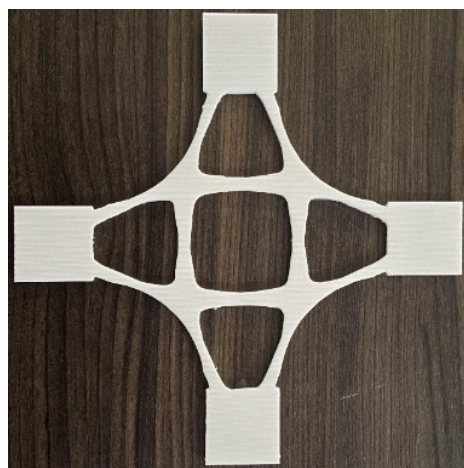
Figure 21. A representative generated model printed using FDM technology.
