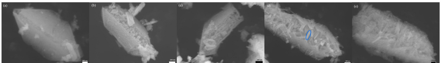
Fig 4. SEM images of the as-prepared CeO 2 products after different reaction time: (a)6h, (b)12h, (c)18h, (d) 24h, (e) 48h, (f) 54h, (g)60h.
