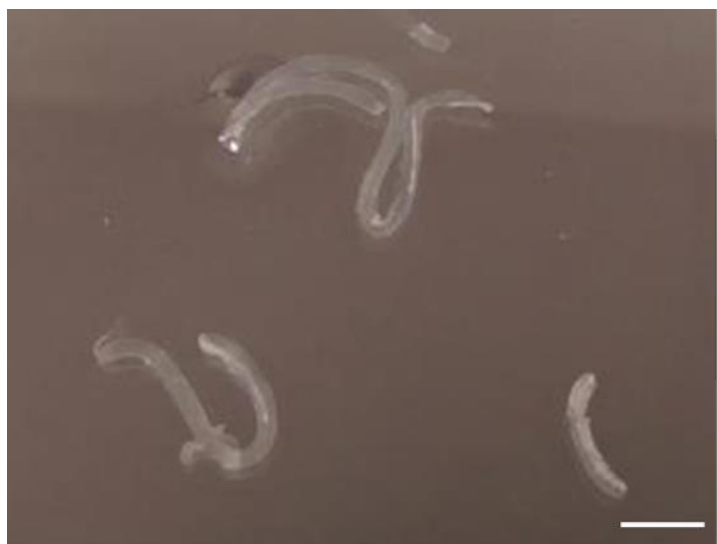
Fig. S5. Retrieval of 1 mm-thick fiber after 4-month transplantation, Related to Figure 4. The fiber was broken into pieces. (Scale bar: 1 cm)
