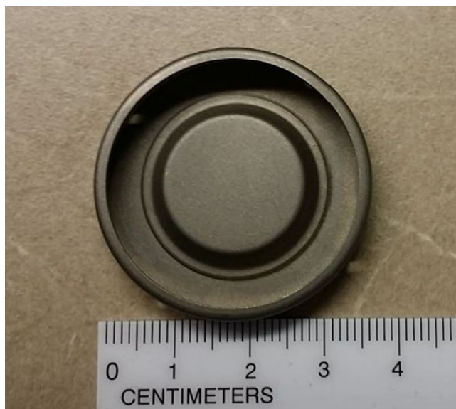
FIG. 1. Image of a typical metallic injection port taken out of a breast tissue expander (ALLERGAN, Santa Barbara, CA).
