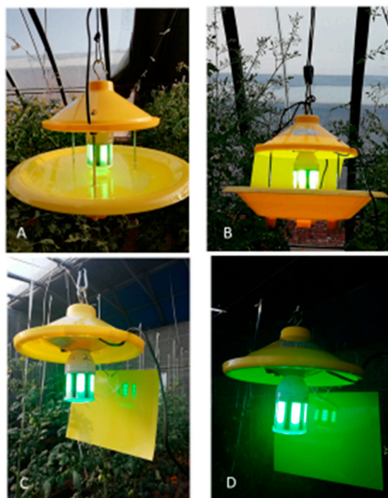
Figure 1. Light emitting diode (LED) traps used in this study. (A) LED water pan trap; (B) LED water pan trap supplemented with a yellow sticky card; (C) LED lit yellow sticky card during the daytime; (D) LED lit yellow sticky card during the nighttime.
