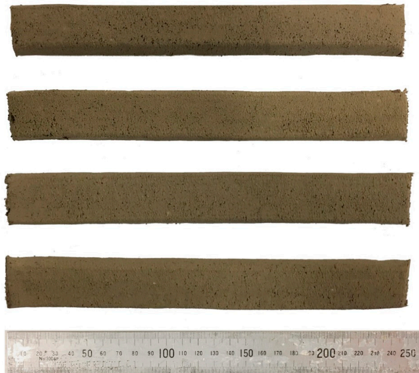
Figure 7. Four 250 mm printed filaments of the “Na-N-2.5” mixture.
