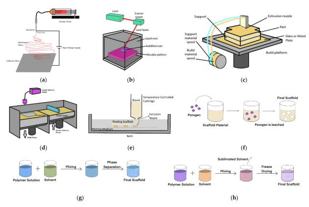
Figure 2. This figure includes schemes of each manufacturing technique manufacturing process. (a) Electrospinning Scheme—Section 4.1; (b) stereolithography or SLA scheme—Section 4.2.1; (c) fused deposition modelling or FDM scheme—Section 4.2.2; (d) selective laser sintering or SLS scheme—Section 4.2.3; (e) bioplotting scheme—Section 4.2.4; (f) salt leaching scheme—Section 4.3; (g) phase separation scheme—Section 4.4; (h) freeze drying—Section 4.5.
