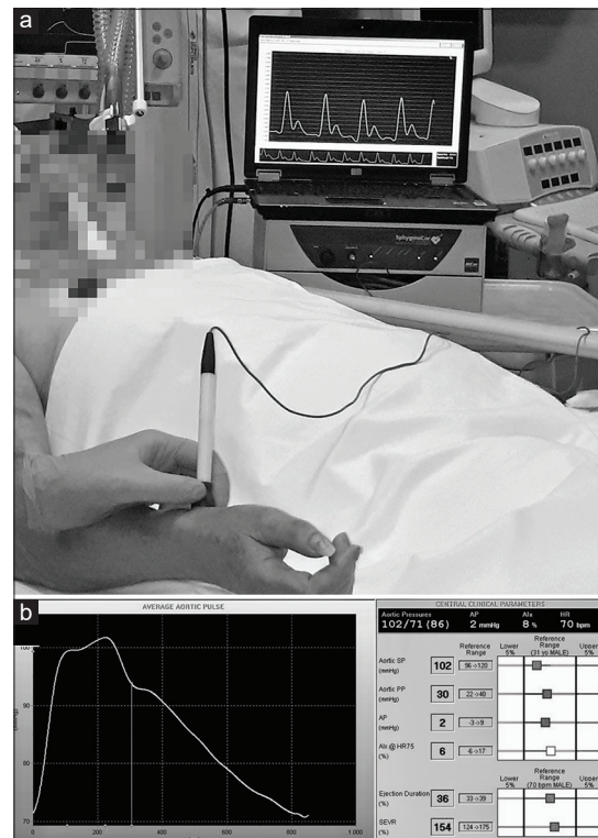
Figure 2: Arterial tonometer. (a) An example of the arterial tonometer (SphygmoCor, AtCor Medical, Sydney, Australia). The monitor shows the noninvasive beat-by-beat analysis of the radial artery pulse wave using applanation tonometry in a patient. (b) In the present layout, the monitor shows the reconstructed aortic arterial pressure wave (left) from a peripheral site and the tonometry-derived values (right) (see text for details)
