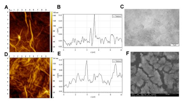
**Figure 1.** Graphene oxide scaffold morphology. (**A**) Atomic force microscopy images and (**B**) a topography model of the surface of the graphene oxide scaffold on a polystyrene culture plate. (**C**) Transmission electron microscopy image of graphene oxide. (**D**) Atomic force microscopy images and (**E**) a topography model of the graphene oxide scaffold surface on a flat silicon wafer. (**F**) Scanning electron microscopy image of the graphene oxide scaffold.
