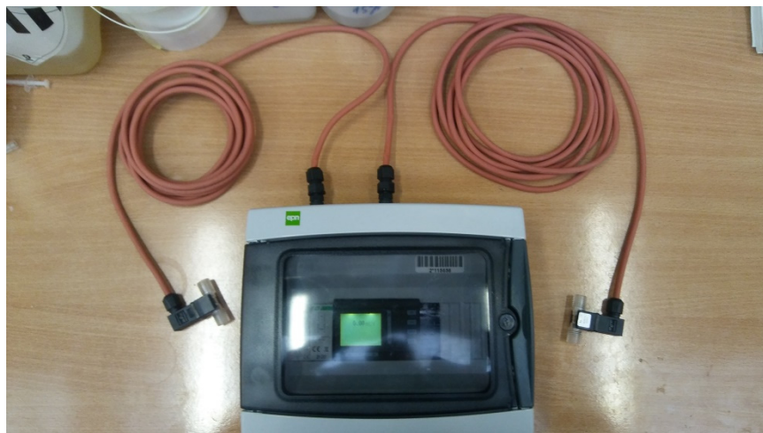
Figure 6. The PLC controller with flow meters.
