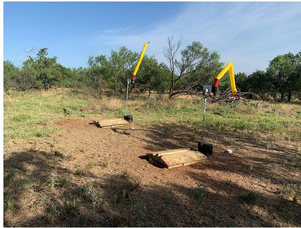
Figure 3. Example of activated deterrent devices (scare dancers) mounted above bait stations containing a sodium nitrite toxic bait in north-central Texas, USA during July 2020. Photo property of USDA.
