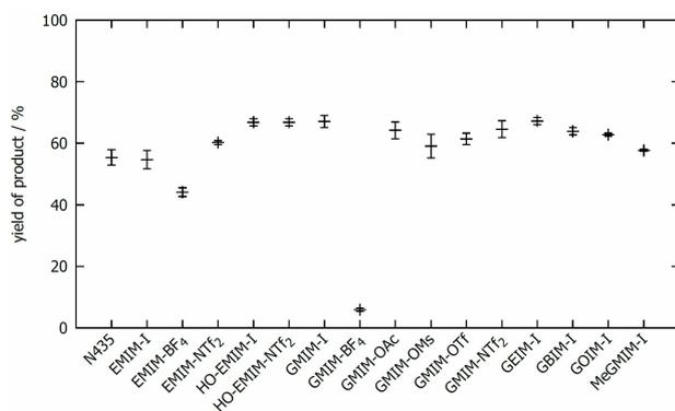
Figure 2. Yield of *n*-butyl acrylate for the reaction of acrylic acid and *n*-butanol with Novozym 435 (N435) and each of the ILs tested in this study. Reaction conditions: 1 mL reaction volume containing acrylic acid (1 M, 1 mmol, 68.6  $\mu\text{L}$ ), *n*-butanol (2 M, 2 mmol, 183  $\mu\text{L}$ ), cyclohexane (748  $\mu\text{L}$ ), N435-biocatalyst (150 mg), 24 h, 25 °C.
