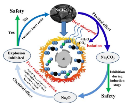
Figure 20. Inhibition process of \text{NaHCO}_3 on aluminum dust.
