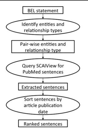
Figure 2. The workflow of the first method employing the semantic search engine SCAIView.
