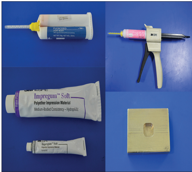
Figure 1: Impression materials and standardized brass mold
