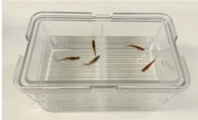
Figure 5. Example of a 1-L Breeding Tank Containing a Separating Barrier between Three Female and Two Male Adult Zebrafish
