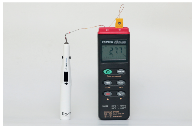
Figure 1. Photograph of a cordless heat plugger connected to a K-type thermometer by a customized copper sleeve.
