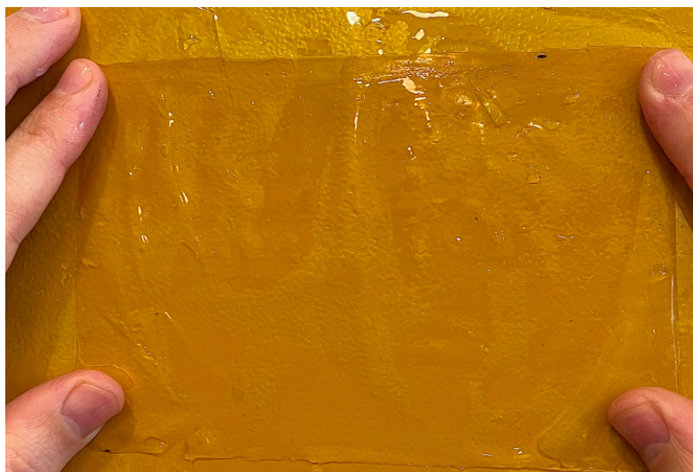
Figure 5. Photograph of a just formed PAN membrane after precipitation and washing with water.
