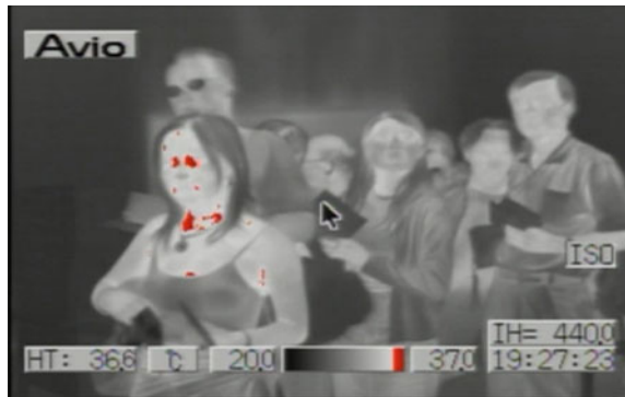
Fig. 1 Isotherm low temperature was set at 35.4 °C, displaying targeting subject in red above the set temperature
