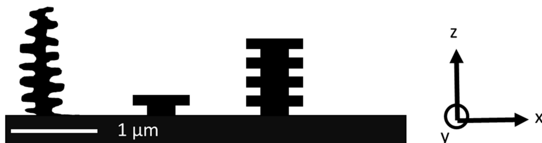
Figure 1. Left: sketch of the cross-section of the nanostructures responsible for the metallic-blue color of the Morpho butterfly. The sketch was created after images found, e.g., in [12,33]. Center and right: model structures used in this work. We started with a single layer “T-structure” and continued to work with the more complex “tree-structure”.
