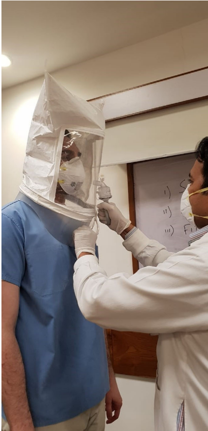
FIGURE 2 Fit test. The previous procedure is repeated with donning N95 respirator and breathing normally, deeply, turning head side to side, up and down, talking and bending over
