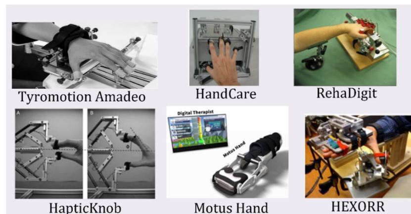
Figure 8. End-effector devices are reviewed in this paper. These devices use end-point control to actuate the hand for proper rehabilitation.
