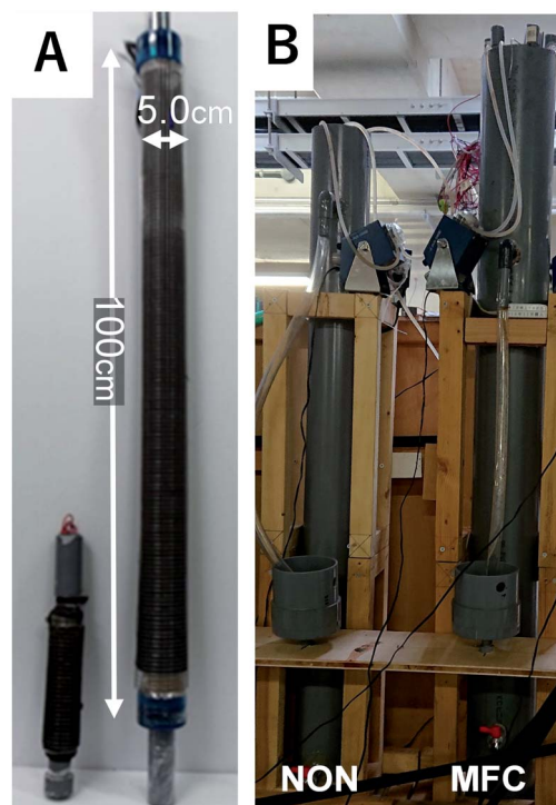
Fig. 1 Appearance of one-meter air-cathode MFC (A) and chemostat reactor without MFC (NON-reactor) and with MFC (MFC-reactor) (B).
