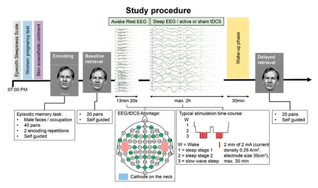
**Figure 3.** Participants underwent this study procedure twice with at least four weeks in between sessions, once with active tDCS and once with sham stimulation. Red rectangles represent anodal tDCS electrodes; the blue rectangle represents the cathodal tDCS electrode. Green shaded circles represent the 22 recording EEG channels overlaid on the 10–20 international electrode system (Fp1, Fp2, F7, F3, Fz, F4, F8, FT9, FT10, C3, Cz, C4, CP5, CP6, P7, P3, Pz, P4, P8, O1, Oz, O2).
