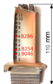
Figure 26. Damaged turbine blades.
