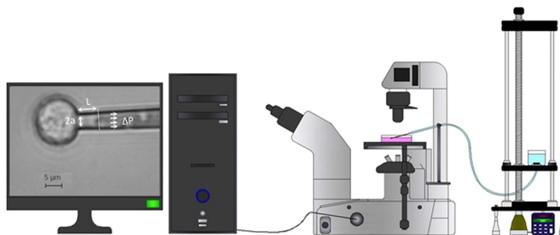
Figure 2. Micropipette aspiration technique was implemented for investigating the mechanical properties of ECs. Desired suction pressure is generated at the end of the micropipette by moving the water reservoir. Generalized Maxwell model's parameters were estimated by dimensions, creep time, applied pressure, and aspirated length.
