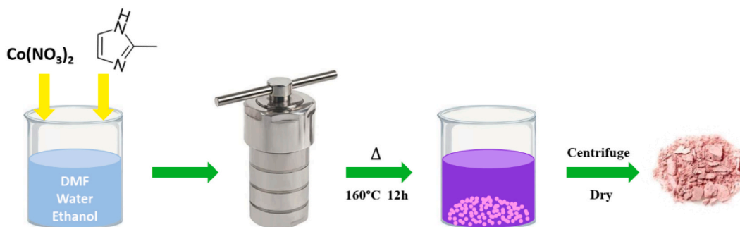
Fig. 2. The schematic of the synthesis procedure for ZIF-67 nanosheets via the hydrothermal method.
