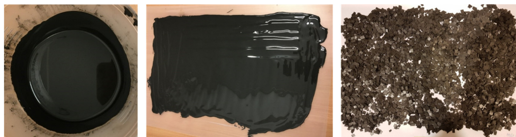
Figure 4. Composites at subsequent stages of fabrication: mixture of polymer, solvent and nickel powder after stirring (left), slurry after pouring on the foil (middle), final composite cut into granules (right).
