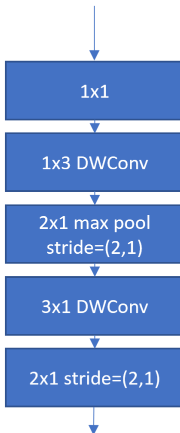
Figure 6. EffNet [5] uses 1 \times 3 and 3 \times 1 depth-wise separable convolutions to reduce model complexity. DWConv denotes depth-wise convolution.
