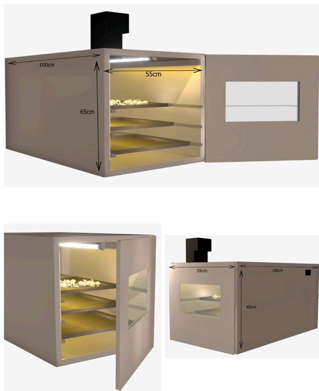
**Fig. 8.** Schematic image of radiant chamber.
