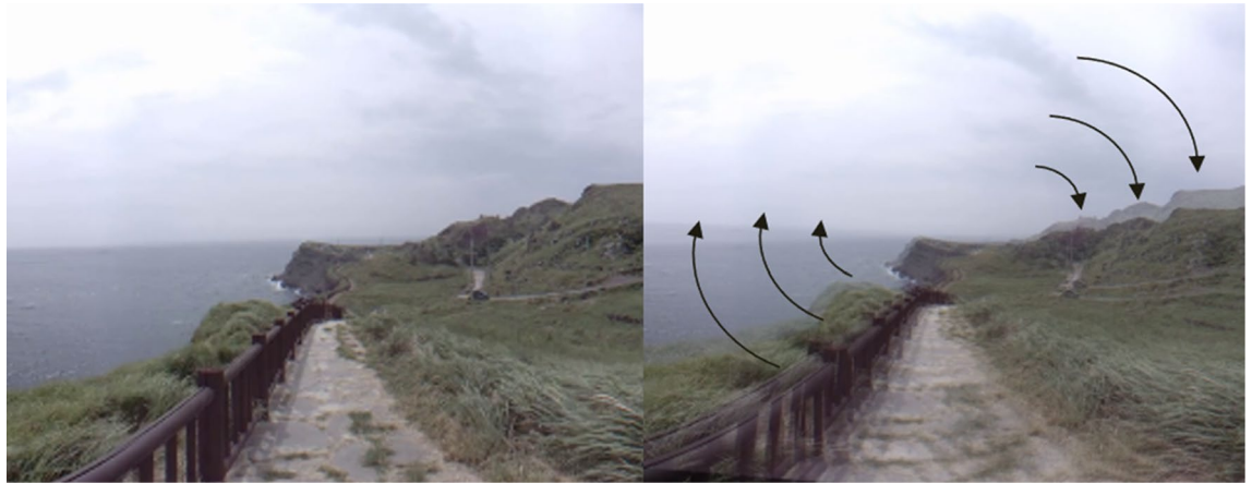
Figure 1. The shaking and dizzy virtual reality (VR) video. The original video (left) was artificially modified for this study by adding a roll swing of the sine waveform at 30 Hz in the Z-axis direction with 0.008^\circ/\text{s} for each grade. Then image movements of 0.3^\circ/\text{s} (VR with less shaking) and 0.38^\circ/\text{s} (VR with more shaking) were made.
