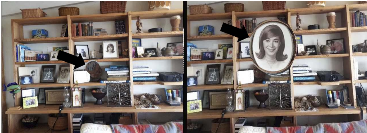
Figure 2. Example of the user-controlled virtual bioptic telescope “magnification bubble.” The image on the left depicts a small sized magnification bubble overlaid on the scene ( arrow ) while the image on the right depicts the result of the user adjusting the size and location of the bubble to a point of interest ( arrow ).
