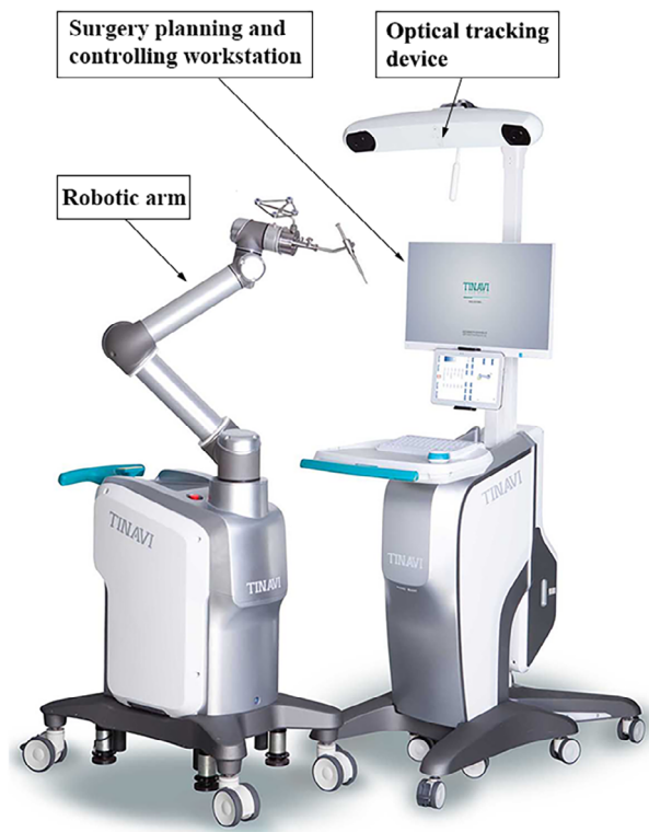
Fig. 1 The TiRobot system. This system consists of an optical tracking device, a surgical planning and controlling workstation, and a surgical robotic arm.
