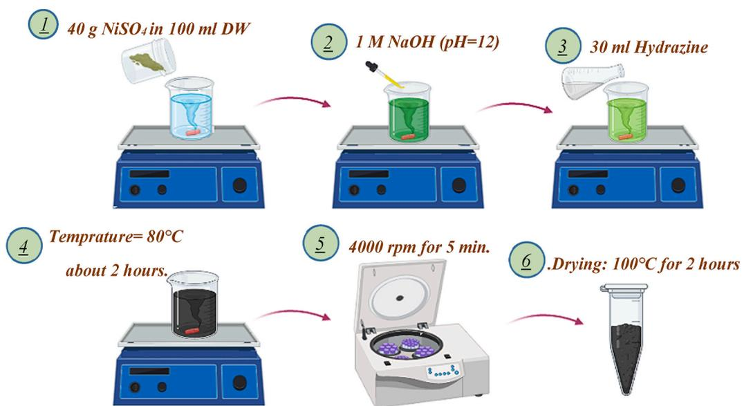
Fig. 1. Nickel synthesis process.
