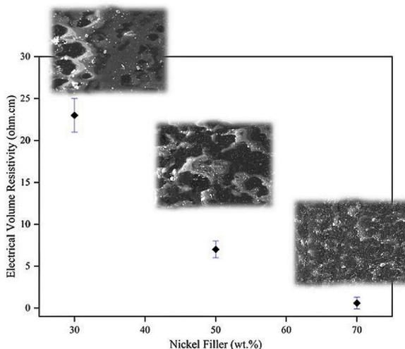
Fig. 5. Variation of volume resistivity of gaskets with the loading of nickel fillers.
