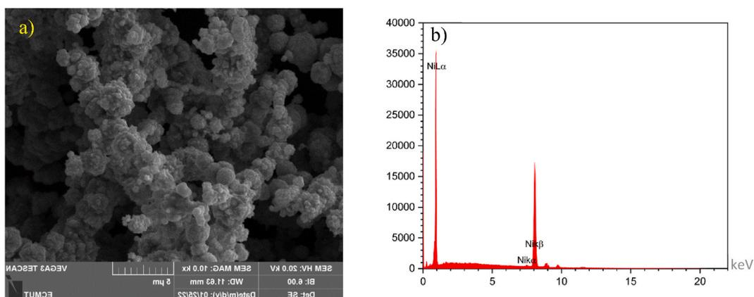
Fig. 3. a) SEM image and b) EDS graph of pure synthesized nickel.
