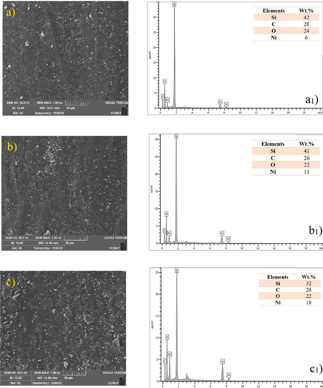
**Fig. 4.** SEM morphology of conductive gaskets, a) 30 wt% filler, b) 50 wt% filler and c) 70 wt% filler and EDS spectrum of samples a<sub>1</sub>) 30 wt% filler, b<sub>1</sub>) 50 wt% filler and c<sub>1</sub>) 70 wt% filler.
