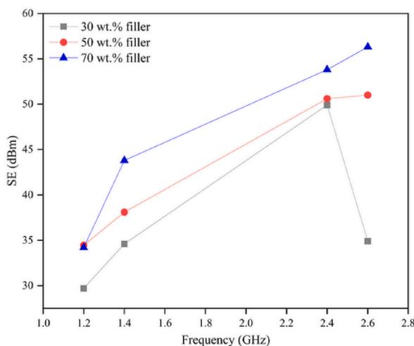
Fig. 6. The shielding effectiveness of gaskets containing different amounts of nickel fillers.
