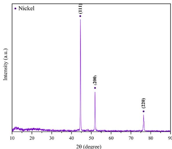
Fig. 2. XRD pattern of pure synthesized nickel.
