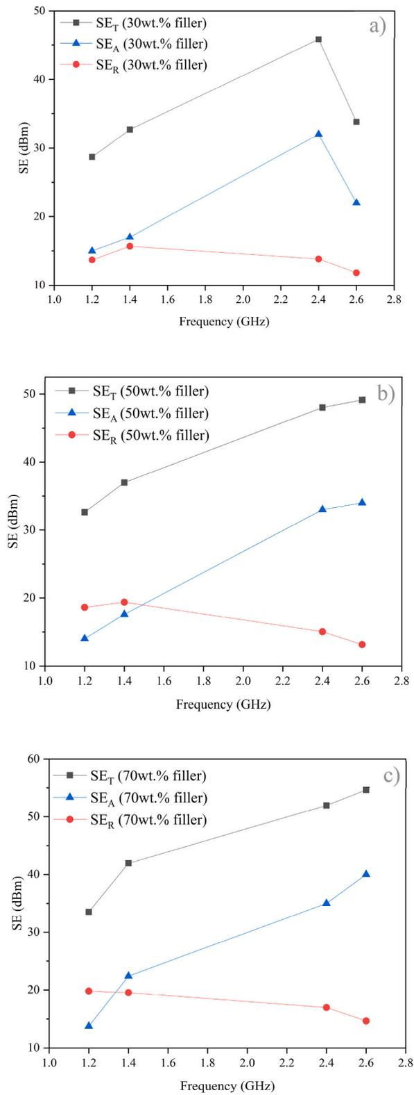
Fig. 7. Shielding results for EMI gaskets (a)  $SE_T$ ,  $SE_A$  and  $SE_R$ , each vs. frequency, a) 30 wt% filler, b) 50 wt% filler and c) 70 wt% filler.
