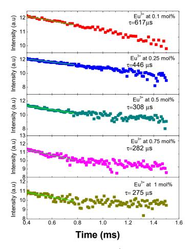
**Figure 6.** Decay curves and lifetimes of  $SiO_2$ -PMMA:Eu<sup>3+</sup> samples with concentration 0.1 mol % (red points), 0.25 mol % (blue points), 0.5 mol % (cyan points), 0.75 mol % (pink points), and 1 mol % (dark yellow points).
