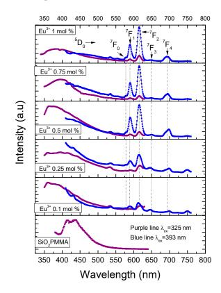
**Figure 4.** Emission spectra after excitation at 325 nm (purple line) and 393 nm (blue line) for the different hybrid material samples. The intensities of the two emission spectra are not at the same scale; they have been normalized to fit into the same plot frame.
