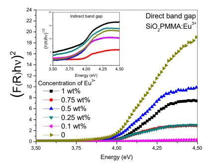
**Figure 2.**  $(F(R)hv)^n$  vs photon energy (Tauc plot) in the absorption edge range for the SiO<sub>2</sub>-PMMA:Eu<sup>3+</sup> samples. In the inset, the  $(F(R)hv)^{1/2}$  vs photon energy relation is plotted for n = 0.5, while in the main graph n = 2.
