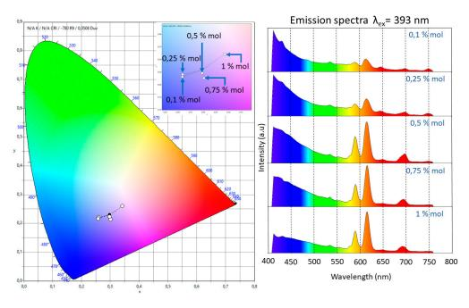
**Figure 5.** CIE 1931 2° chromaticity diagram. Color chromaticity of the emission in the range of 410–760 nm of the five doped samples under the excitation wavelength at 393 nm. The inset in the diagram represents an amplification of the blue-pale red zone. The red shift in the emission was observed as an increase of the molar relation of  $Eu^{3+}$ .
