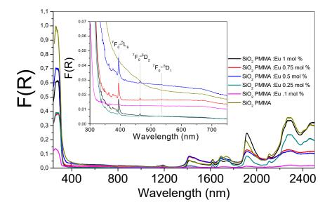
**Figure 1.** Absorption spectra of the six  $SiO_2$ - methyl methacrylate (PMMA) samples. The absorption spectra for the undoped and doped hybrid samples are shown in the wavelength range between 240 and 2500 nm. In the inset, a zoom of the range 300–750 nm is presented, where the electronic transitions of the Eu<sup>3+</sup> ion are identified. The line color of each sample is the same in both graphs.
