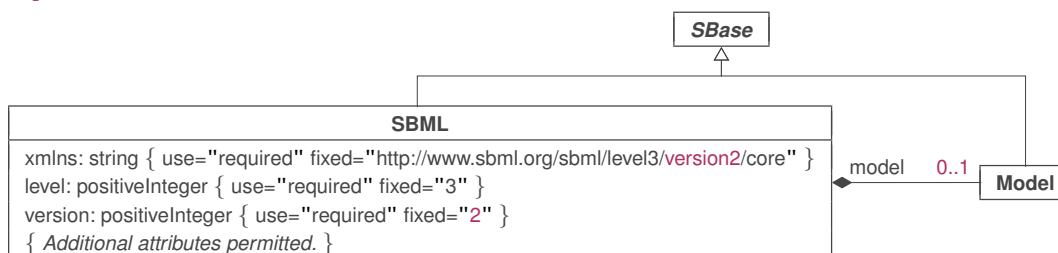
Figure 9: The definition of class SBML for SBML Level 3 Version 2 Core. The class Model is defined in Section 4.2 on p. 35. Note that SBML and Model are subclasses of SBase , and therefore inherit the attributes of that abstract class.
