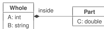
Figure 2: Example illustrating composition: the definition of one class of objects employing another class of objects in a part-whole relationship. In this particular example, an instance of a Whole class object must contain exactly one instance of a Part class object, and the label referring to the Part class object is inside . In XML, this symbol becomes the name of a subelement and the content of the subelement follows the definition of Part .
