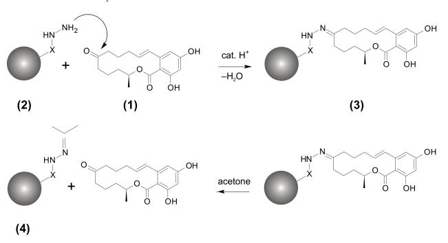
**Figure 1.** Concept of reversible covalent hydrazine chemistry (RCHC): Zearalenone (ZEN) (1) is extracted from oil sample by reaction with the hydrazine moiety linked to a solid phase (2) to form ZEN-hydrazone (3), which can be cleaved into ZEN after removal of matrix compounds. The acetone-loaded solid phase (4) can be re-activated to (2) for its reuse.
