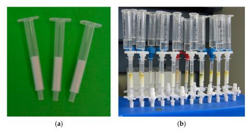
**Figure 2.** (a) RCHC-SPE cartridges: 1 mL PP cartridges filled with 400  $\pm$  2 mg hydrazine-functionalized material SC-1; (b) RCHC-SPE cartridges in use for extraction and clean-up of ZEN from edible vegetable oils.
