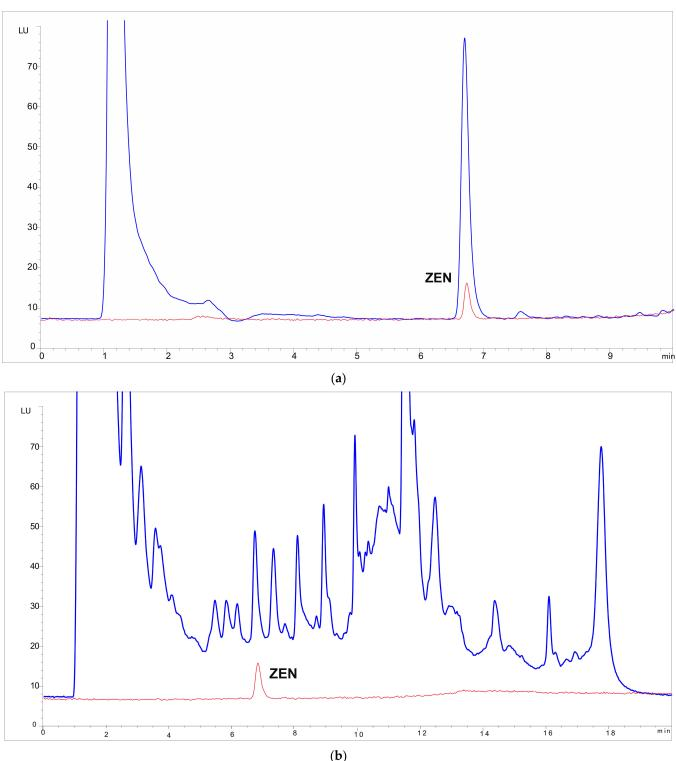
**Figure 4.** Blue lines: HPLC-FLD chromatograms of the native wheat oil sample-No. 5 from interlaboratory comparison study containing 494  $\mu g/kg$  ZEN; red lines: ZEN standard solution in acetonitrile (60 ng/mL). Sample preparation according to (a) RCHC-SPE method with hydrazine-functionalized material SC-1, and (b) official standard method EN 16924:2017 (HPLC-FLD part).
