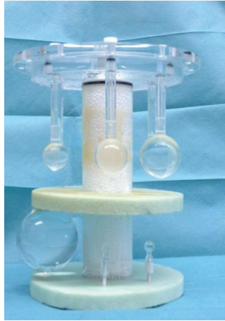
FIGURE 1: Inserts in the IEC phantom used for the multicenter measurements comprising 9 fillable spheres of different diameters.
