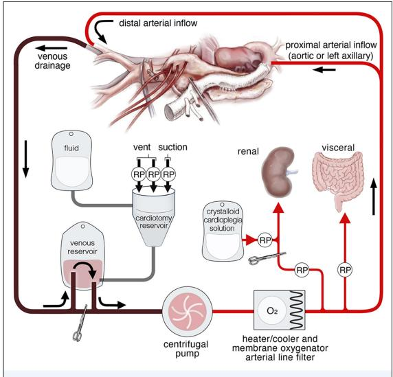
FIGURE 2 Modified cardiopulmonary bypass circuit in full cardiopulmonary bypass configuration. Inflow and outflow clamps are removed, and a clamp is replaced across the reservoir bypass line. Venous drainage is diverted into the venous reservoir. For full conversion to cardiopulmonary bypass, the surgeon places a long venous cannula for right atrial drainage and a proximal arterial inflow (aortic or axillary). (RP, roller pump.)
