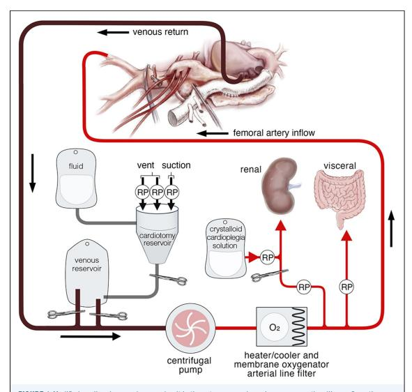
FIGURE 1 Modified cardiopulmonary bypass circuit in the extracorporeal membrane oxygenation-like configuration. Reservoir is isolated from circuit by 2 line-clamps at the venous reservoir inflow and outflow. Venous drainage flows directly onward to the centrifugal pump. During venoarterial extracorporeal membrane oxygenation mode, volume from the reservoir may be added to the circuit by temporarily removing the reservoir outflow clamp. (RP, roller pump.)
