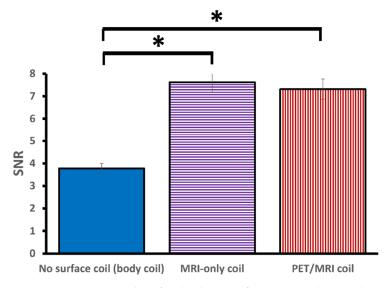
**Figure 6.** Mean SNR values for the three configurations. The error bars represent the standard error. PET/MRI and MRI-only showed significantly higher SNR values as compared to the configuration without a surface coil. No significant difference in SNR was observed between PET/MRI and MRI-only coils. The asterisks ("\*") indicate a significant difference in SNR (p < 0.05).
