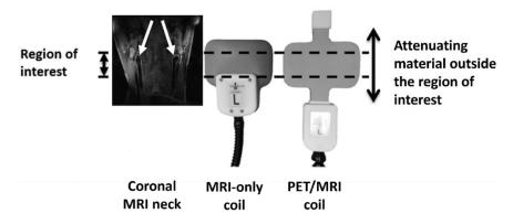
**Figure 1.** Adaptations to the design of the PET/MRI coil. For the dedicated PET/MRI coil, the electronic housing has been moved further away from the coil elements. The cushioning material that has been used is also thinner and less attenuating. The white arrows point to the left and right carotid arteries.
