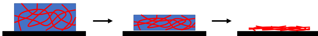
Figure 1. Simplified cartoon showing the collapse of a 3D network to a 2D film on drying.
