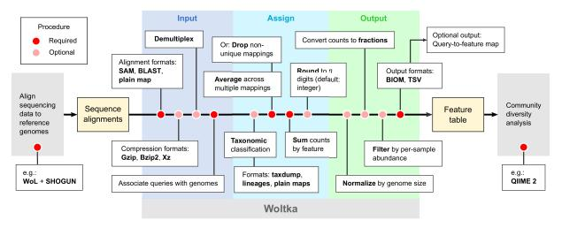
**FIG 9** Procedure for generating OGU tables, as implemented in Woltka. This program serves as an interface connecting upstream sequence alignment and downstream community diversity analysis. The inputs are sequence alignments, and the outputs are feature tables (in this case, OGU tables). The pipeline contains multiple procedures, with rich format support and flexible options to address diverse user needs.
