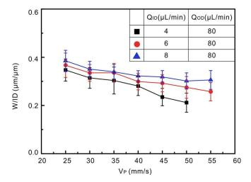
**Figure 7.** Trace widths normalized by ID as a function of the platform speed. Three different ratios of  $Q_{ID}/Q_{OD}$  were used for study (ID = 210  $\mu$ m, OD = 800  $\mu$ m). There is no continuously trace when the moving speed is over 50 for small liquid alloy flow rate (black squares).
