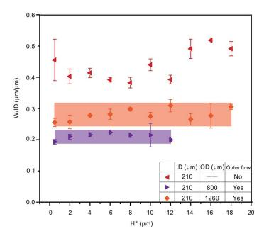
**Figure 5.** Trace widths normalized by ID as a function of H\* and 95% confidence interval of widths printed by CNINE. A uniaxial nozzle and two CNINE with different outer channel diameters were used for the study ( $Q_{ID} = 8 \mu L/min$ ,  $V_P = 40 \text{ mm/s}$ ). H\* is the relative distance between the outlet of coaxial nozzle and its baseline (H\* = H – 5  $\mu$ m).
