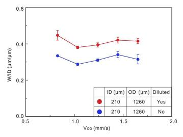
**Figure 8.** Trace widths normalized by ID as a function of outer channel flow speed with and without diluted outer flow ( $Q_{1D} = 8 \mu L/min$ ,  $V_P = 40 \text{ mm/s}$ ).
