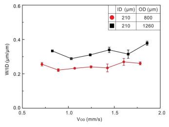
**Figure 6.** Trace widths normalized by ID as a function of outer channel flow speed. Two CNINE with different outer channel diameters were used ( $Q_{\rm ID}$  = 8  $\mu$ L/min,  $V_{\rm P}$  = 40 mm/s).
