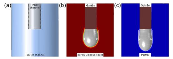
**Figure 3.** Simulated behavior of liquid alloy in the coaxial nozzle. (a) The model of flow field; (b) simulated behavior of liquid alloy with a purely viscous outer flow with the same viscosity as the PDMS; (c) simulated behavior of liquid alloy with PDMS squeezing. The flow rates of GaInSn and outer channel flow are  $16~\mu L/min$  and  $80~\mu L/min$ , respectively. The diameters of the inner channel and outer channel are  $210~\mu m$  and  $800~\mu m$ , respectively.
