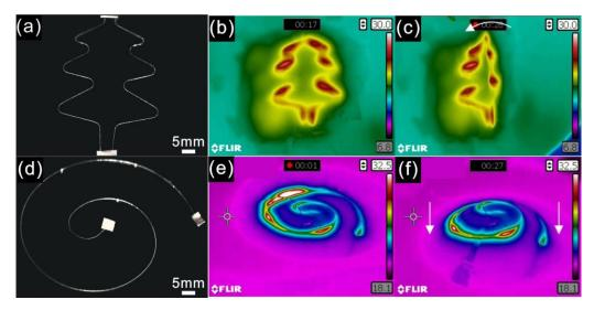
**Figure 11.** Printed structures with different diameters of liquid alloy: (a) printed tree structure heating device; (b) infrared thermography of tree structure heating device when applied voltage is 2 V; (c) infrared thermography of tree structure heating device after bending 90°; (d) helix structure heating device; (e) infrared thermography of helix structure heating device when the applied voltage is 2.5 V; (f) infrared thermography of helix structure heating device after stretching.
