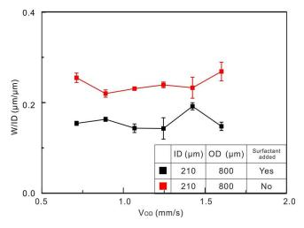
**Figure 9.** Trace widths normalized by ID as a function of outer channel flow speed with and without surfactant added outer flow ( $Q_{\rm ID}$  = 8  $\mu$ L/min,  $V_{\rm P}$  = 40 mm/s).
