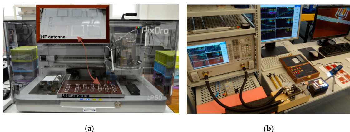
Figure 9. The ink-jet printed flexible antenna: (a) UHF and HF tag antennas under manufacturing process; (b) HF tag antenna under tests.
