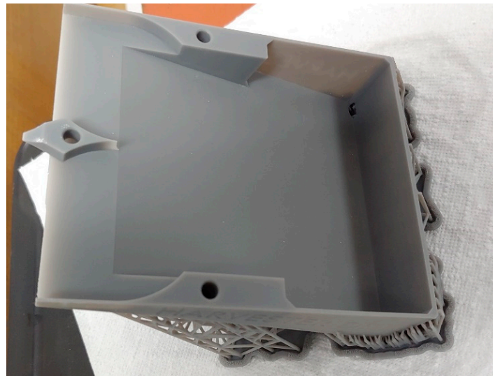
Figure 7. Harvester main body produced using the SLA method.
