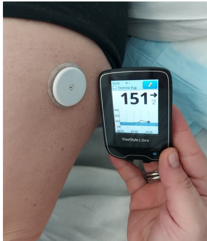
Figure 2. The sensor is applied to the arm of a patient with a subcutaneous needle measuring interstitial glucose levels. Measurements are viewed on a receiver unit (either a smartphone or dedicated receiver unit). This model is a FreeStyle Libre.
