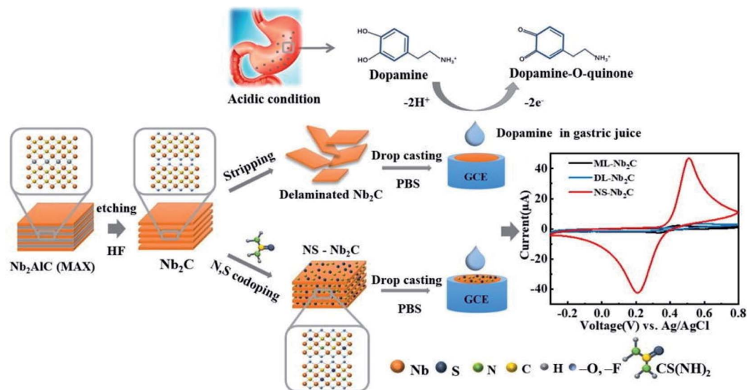
Fig. 10 Schematic synthesis of N,S co-doped \text{Nb}_2\text{C} MXene and assembly for DA sensing in acidic condition. CV curves on the right side shows that the redox current peaks in case of N,S co-doped \text{Nb}_2\text{C} sheets are greatly enhanced as compared to multilayered (ML) or delaminated (DL) \text{Nb}_2\text{C} MXene. Due to high electron transfer rate and surface area expansion for molecular interaction imparted by N,S doping. Reproduced from ref. 178 after permission, copyright© 2021 Elsevier.
